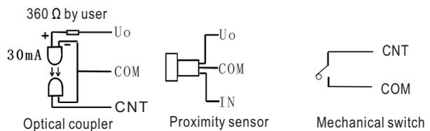
1. Proximity sensor wiring above is for NPN type sensor. Add a 1kohm resistor between IN and COM for PNP type sensor.
