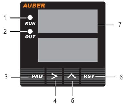
1. RUN LED. Flashing during delay, cumulating or counting. Stay on in other conditions.
