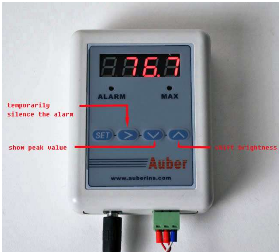
Figure 2 Function keys during temperature measurement operation
