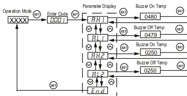
Figure 4. Flow chart of how to set the alarm
