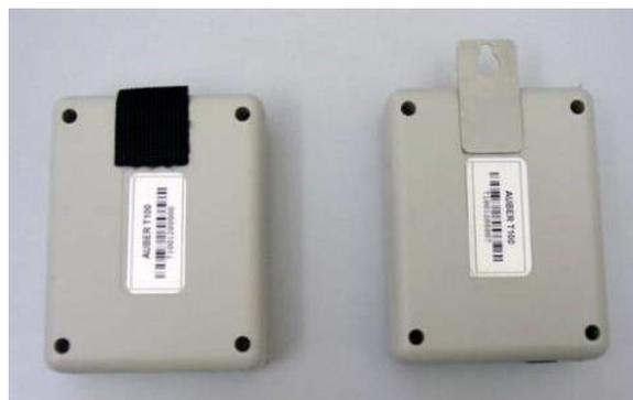
Figure 6. Left, using Velcro for mounting. Right, using stainless steel plate for mounting.
