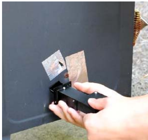
Figure 4. Insert the spring to the hole
