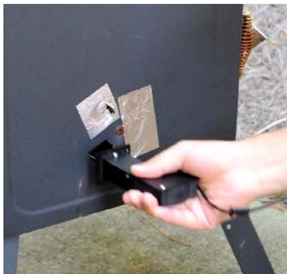
Figure 6. Pull the blower out with one hand
