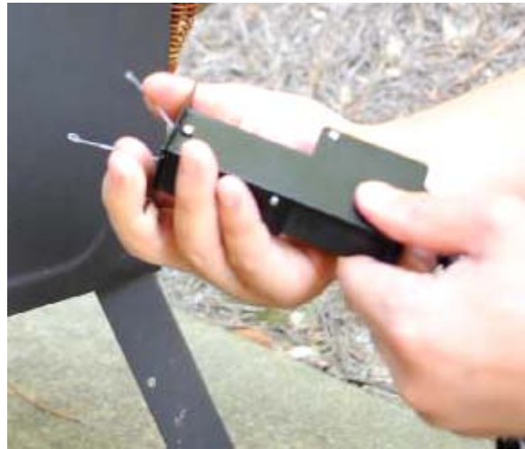
Figure 3. Squeeze the spring
