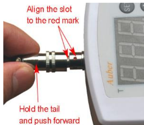
Figure 5. Install the Sensor.
