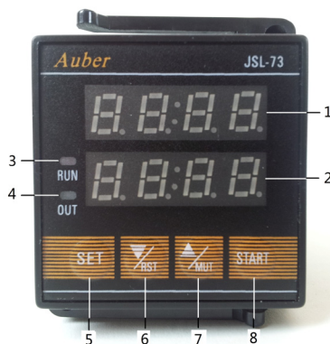
Figure 1. Front panel of JSL-73C-24 timer.
