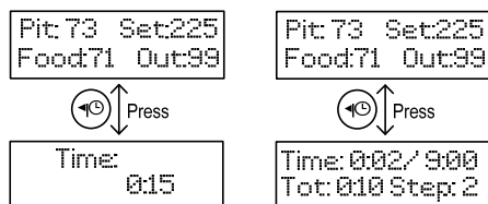
Figure 4. Using Timer/Back key to check cooking time in single-step mode (left) and in multi-step mode (right).
