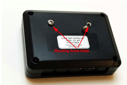
Figure 14. Two M4 screw holes on the back of the controller.
