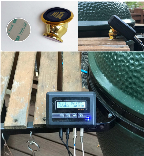
Figure 15. Holding the controller by smartphone magnetic mounting stands. This type of stand has double-sided tape at the bottom. The tape may not stick to the weathered wood. Epoxy was used to hold the stand in this picture.
