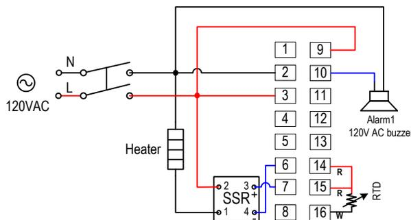
Figure 8. SYL-4352 or SYL-4352P with RTD input. This is a typical wiring for controlling the temperature of a tank of liquid with high precision.
