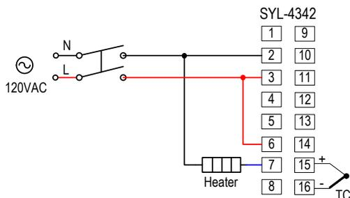
Figure 6. SYL-4342 or SYL-4342P control the heater directly by the internal relay of the controller. The heater must consume less current than the internal relay's maximum rating (7A at 240V AC and 10A at 120V AC).
