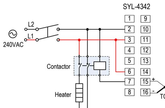
Figure 7.2. SYL-4342 or SYL-4342P with thermocouple input and external relay output for 240VAC system.
