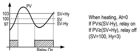
Figure 5. On/off control mode
