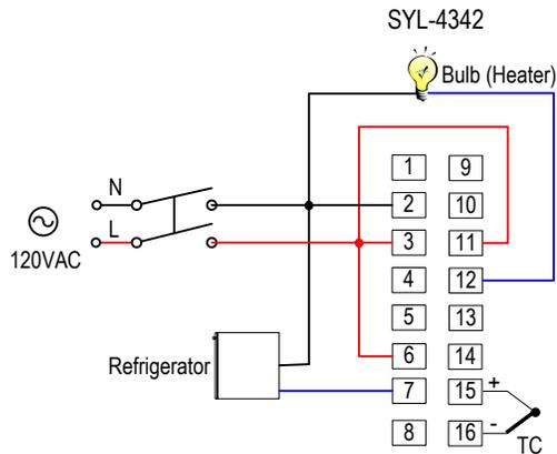
Figure 11. A refrigerator connected to SYL-4342 directly
