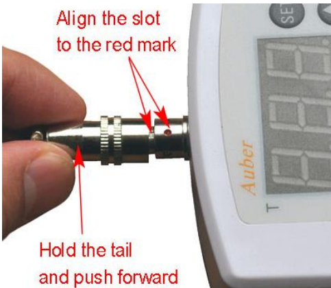
Figure 3. Install the Sensor
