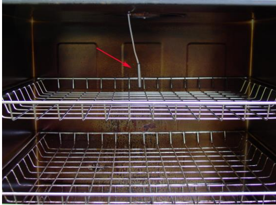
Fig 5. Sensor position. Left, the sensor should be placed close to the food but high enough so that it does not touch the food. Right, hold the sensor in place with a piece of tape.
