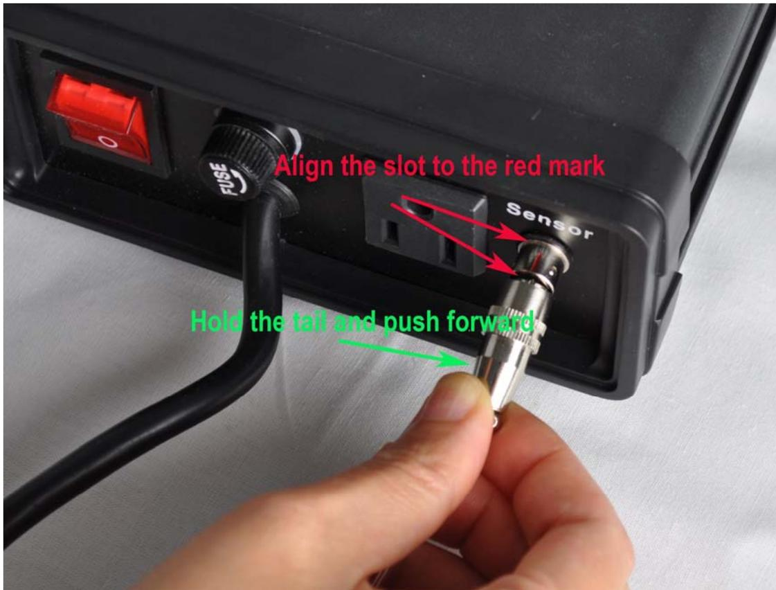
Fig 3a. How to install the sensor.
