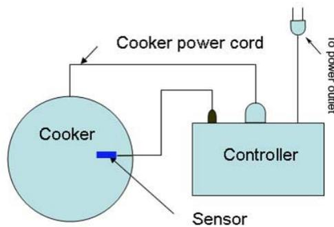
Figure 3. Typical connection between the controller and the heating device (in this example, the cooker).
