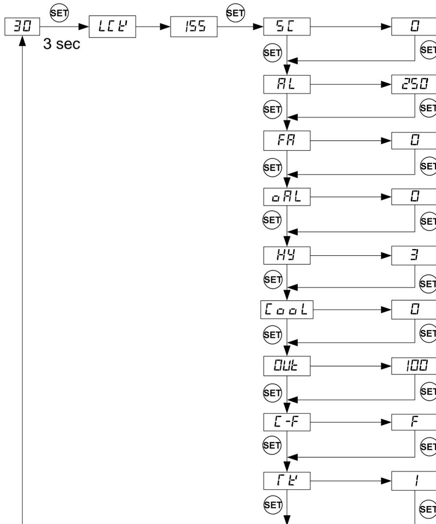
**Figure 5. Code 155 Parameter setup flow chart**
