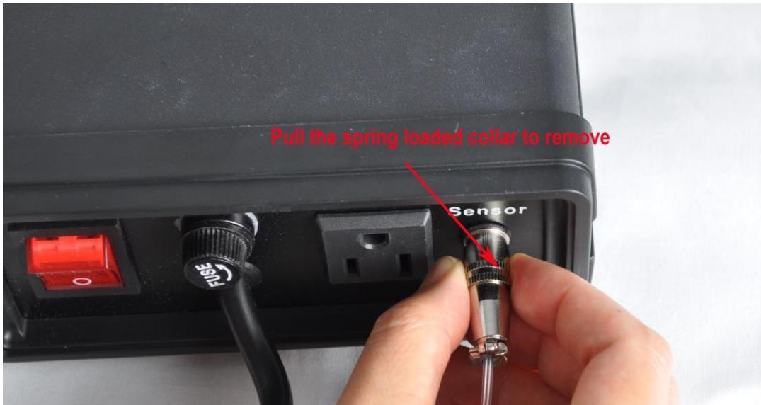
Fig 3b. How to remove the sensor.
