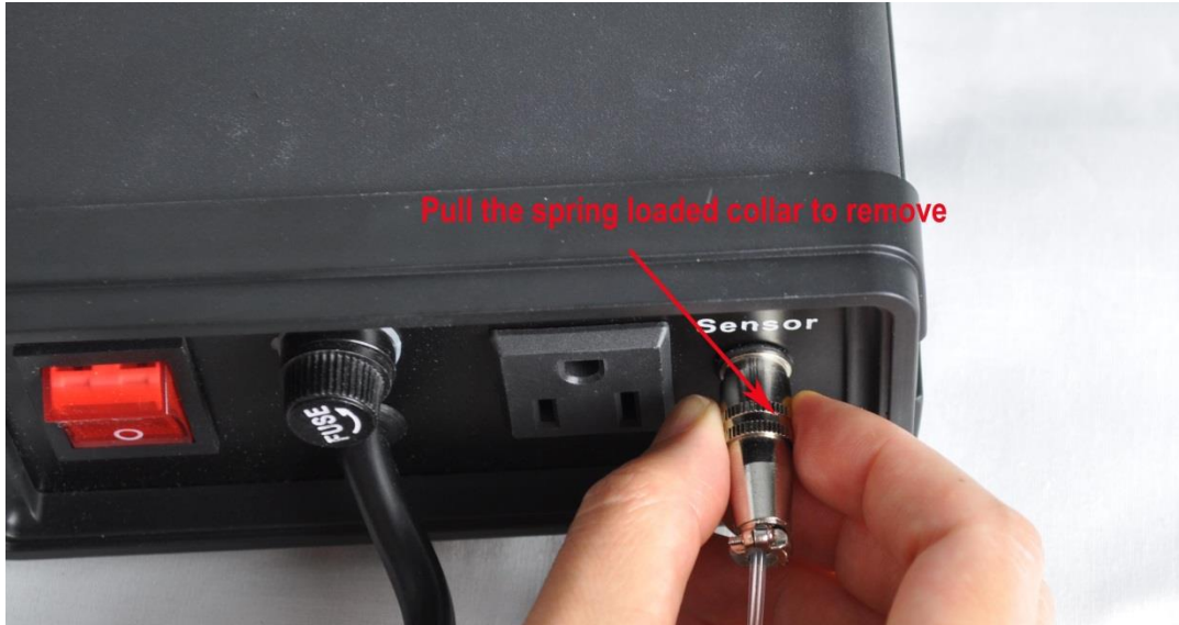
Figure 4. How to remove the sensor.
