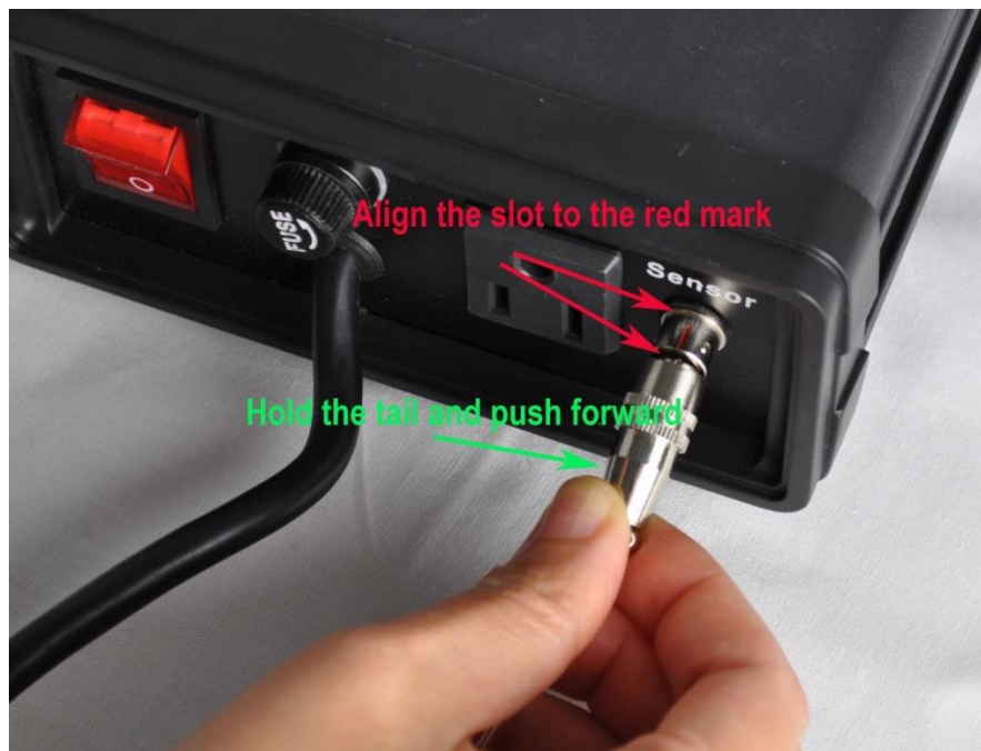
Figure 3. How to install the sensor.
