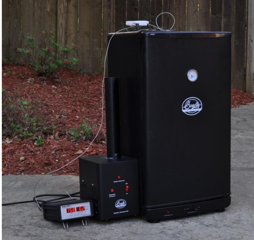
Figure 7. Connection between the controller and smoker
