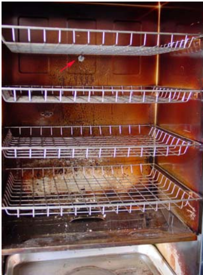
Fig 1, Inside view. Red arrow points to the sensor. It should be installed close to the top cooking rack but not touch it. It could interfere with the food on the second rack if it is lower than that position.
