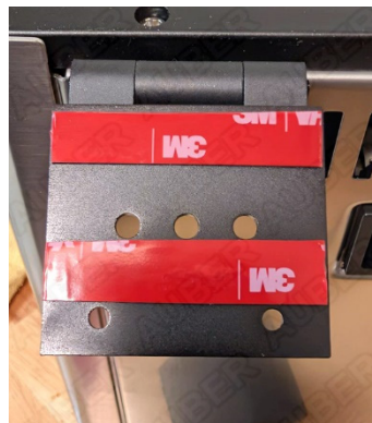
Figure 4. Apply double-sided tape to the top plate.
