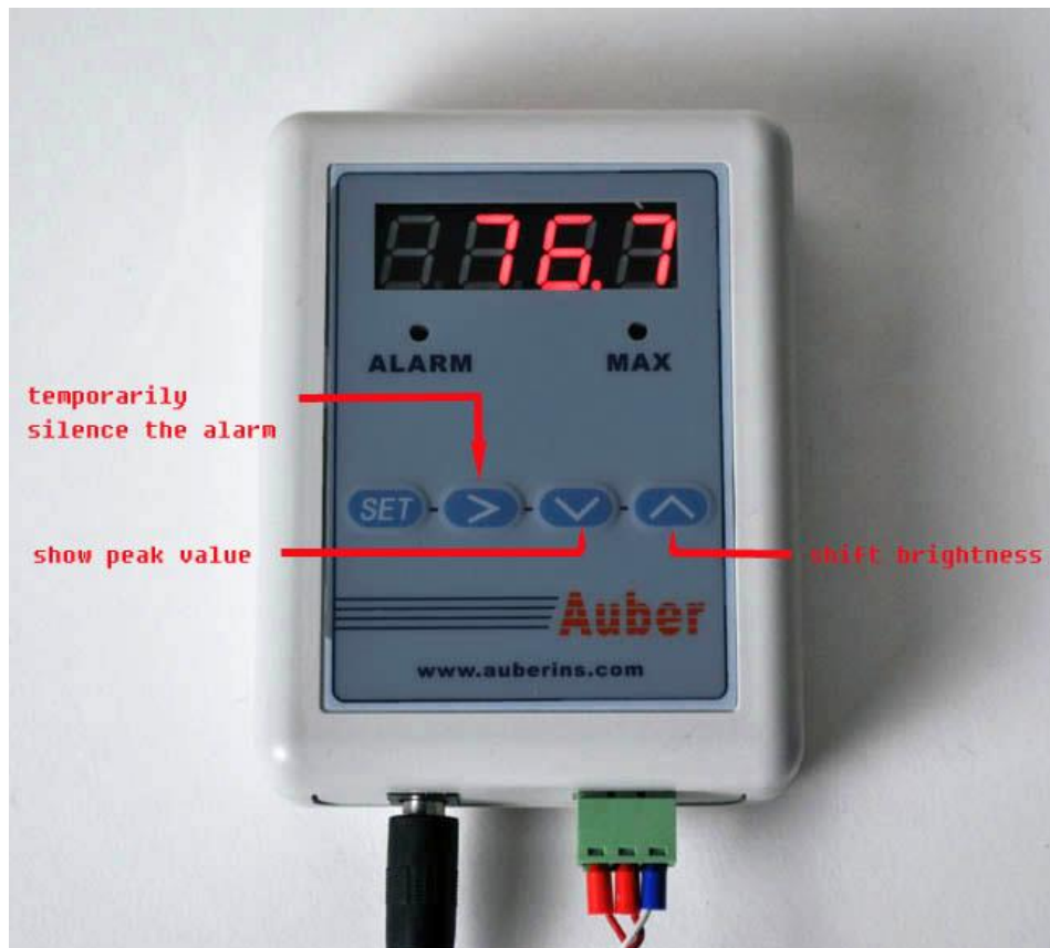
Figure 2 Function keys during temperature measurement operation
