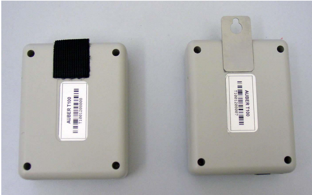
Fig 6. Left, using Velcro for mounting. Right, using stainless steel plate for mounting.
