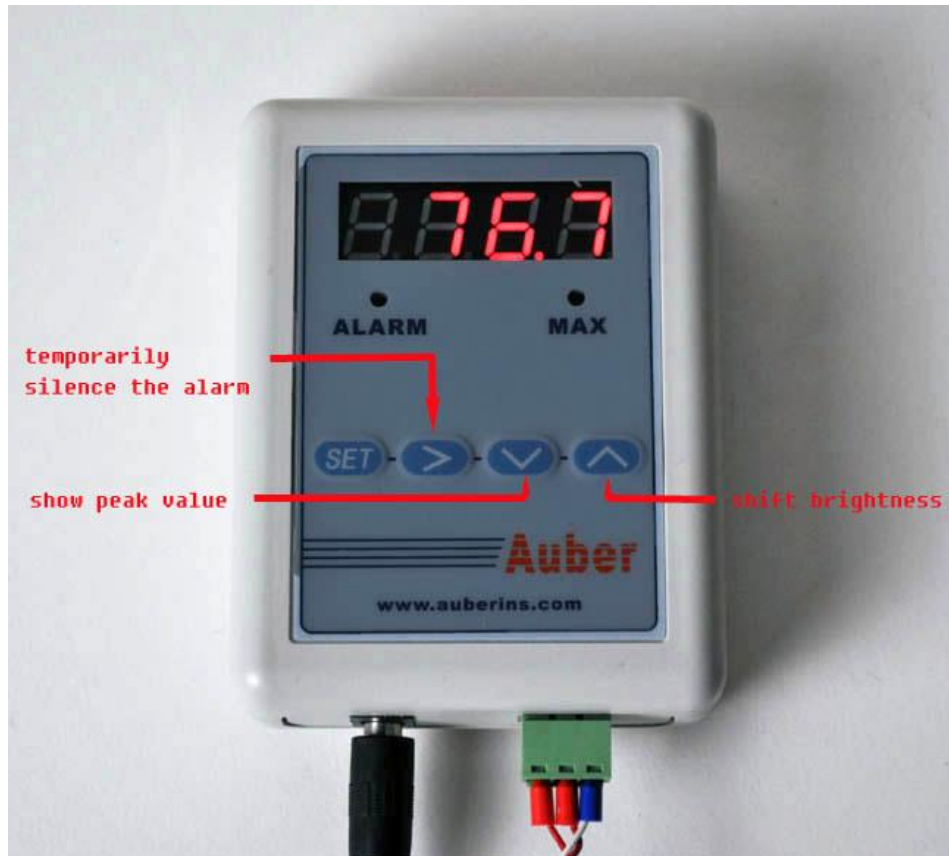
Figure 2. Function keys during temperature measurement operation
