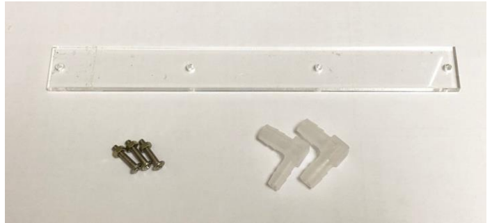
Figure 6. Clear extension arm for supporting arm (top), three pairs of screws and nuts to mount the extension arm (lower left), and two dispensing nozzles (lower right).
