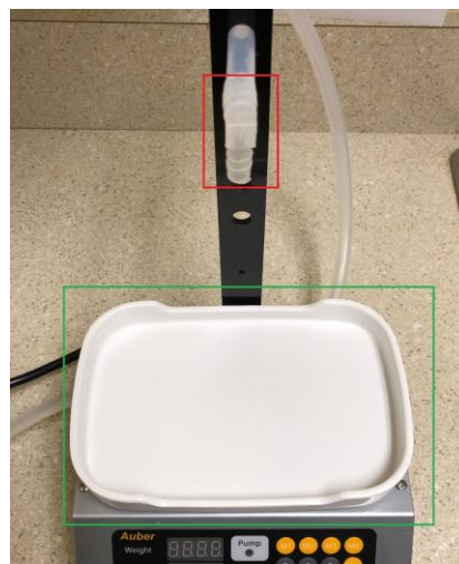
Figure 11. Nozzle at end of the outlet pipe (highlighted in red). White tray over the black measuring board (highlighted in green)
