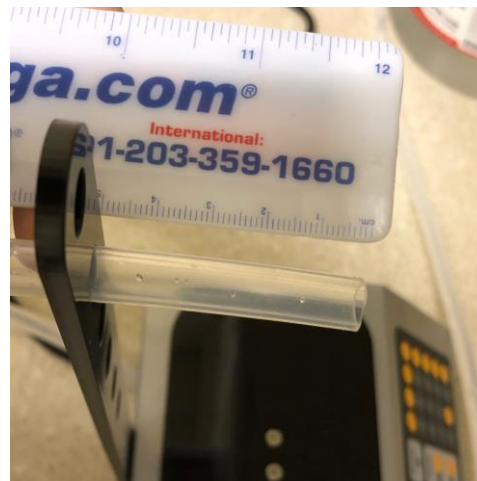
Figure 10. 2-inch distance between the supporting arm and pipe end.
