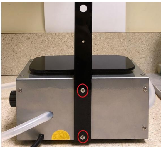
Figure 8. Supporting arm installed.
