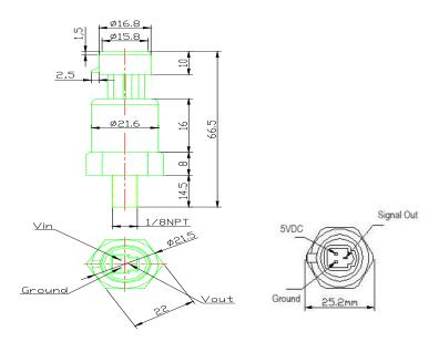
This pressure transmitter is to be powered by regulated 5 VDC power supply. Connect Red (or Brown) wire to the 5VDC power source. Connect black wire to the ground. Green or (Blue) wire is the signal output.
