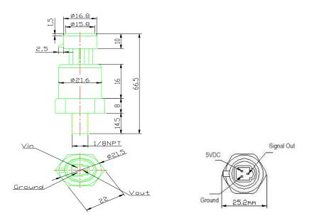
This pressure transmitter is to be powered by regulated 5 VDC power supply. Connect Red (or Brown) wire to the 5VDC power source. Connect black wire to the ground. Green (or Blue) wire is the signal output.
