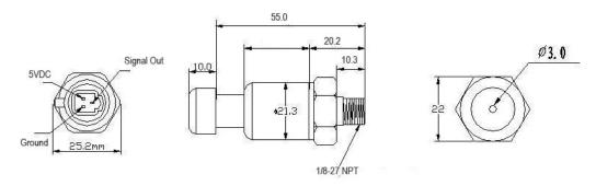
Dimension in drawing is in millimeters, except the thread.
