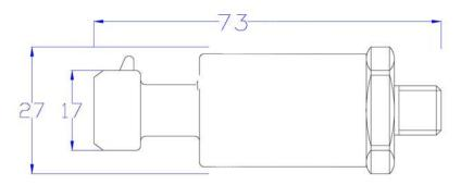
This pressure transmitter is to be powered by regulated 5 VDC power supply. Connect red wire to the 5VDC power source. Connect green wire to the ground. Yellow wire is the signal output.
