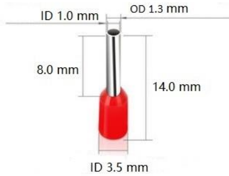
E0508 Ferrule (Cable size:0.5mm, fit 22 AWG wire).
