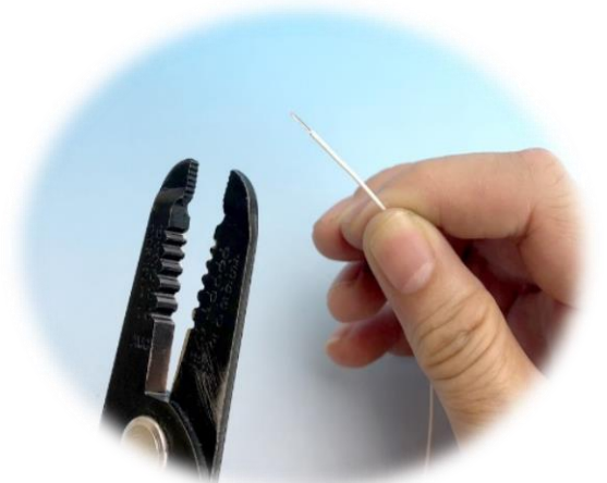
Select the right crimp slot to strip the wire.
