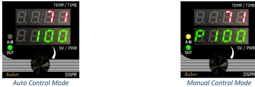
Figure 3. A DSPR-5 controller in Auto Control Mode with the SV set at 100°F (left) and the controller in Manual Control Mode with the SV set at 100% output (right).
