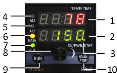
Figure 1. The front panel of DSPR320.
