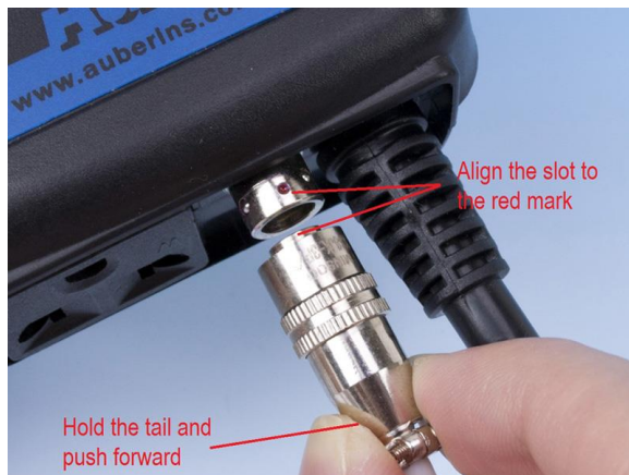
Figure 3. Install the Sensor.
