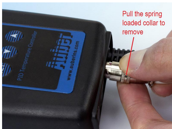
Figure 4. Remove the Sensor.
