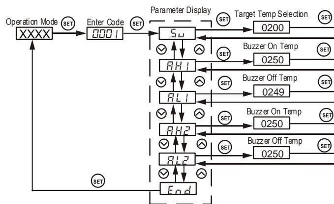
Figure 2. Flow chart for how to set target temperature and alarm.
