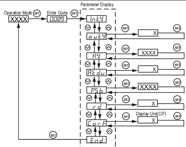
Figure 6. The system setup flow chart
