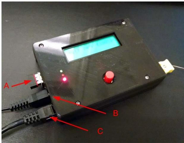
Figure 1. Plug a wireless adapter to the USB port on Raspberry Pi indicated by red arrow A. The arrow B and C are the power input plug and the output cable to blower.
