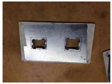
6) Using the jig saw to carefully trim off the extra metal. Then, use the file to do the final adjustment. Drill the center hole for the connector.
