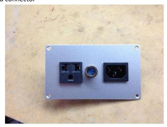
9) If the components are not snap tight, use a little hot melt glue on the inner side will solve the problem.
