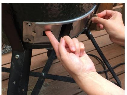
Figure 3(a). Lift the adapter plate so both edges are in the groove.
