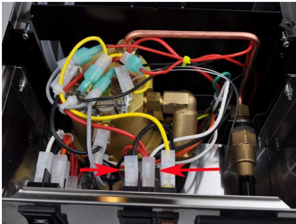
Figure 10. Red arrow indicates the connectors that controller power cable will be tapped.
