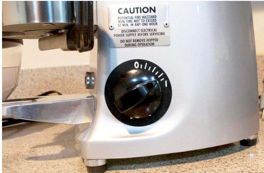
Step 3. Install the nub back. First align the pointer of the nub to the "O" on the dial. Push the nub half way onto the switch shaft. Then rotate the nub to "I" position and press the nub all the way in until it contacts the tape. The nub should be stopped between O and I position by the tape.
