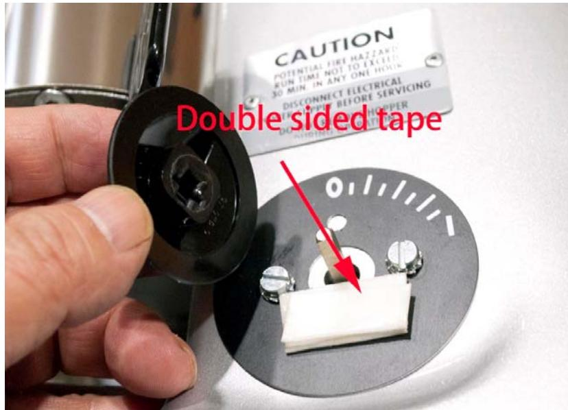
Step 2. Apply three layers of double sided tape. Three layers are needed to build up enough thickness so that they will stick to the rim of the switch nub. The position of the
