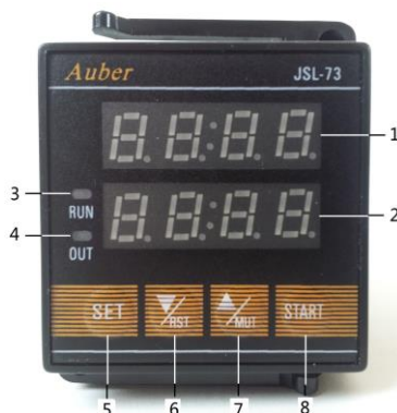
Figure1. Front panel of JSL-73B timer.
