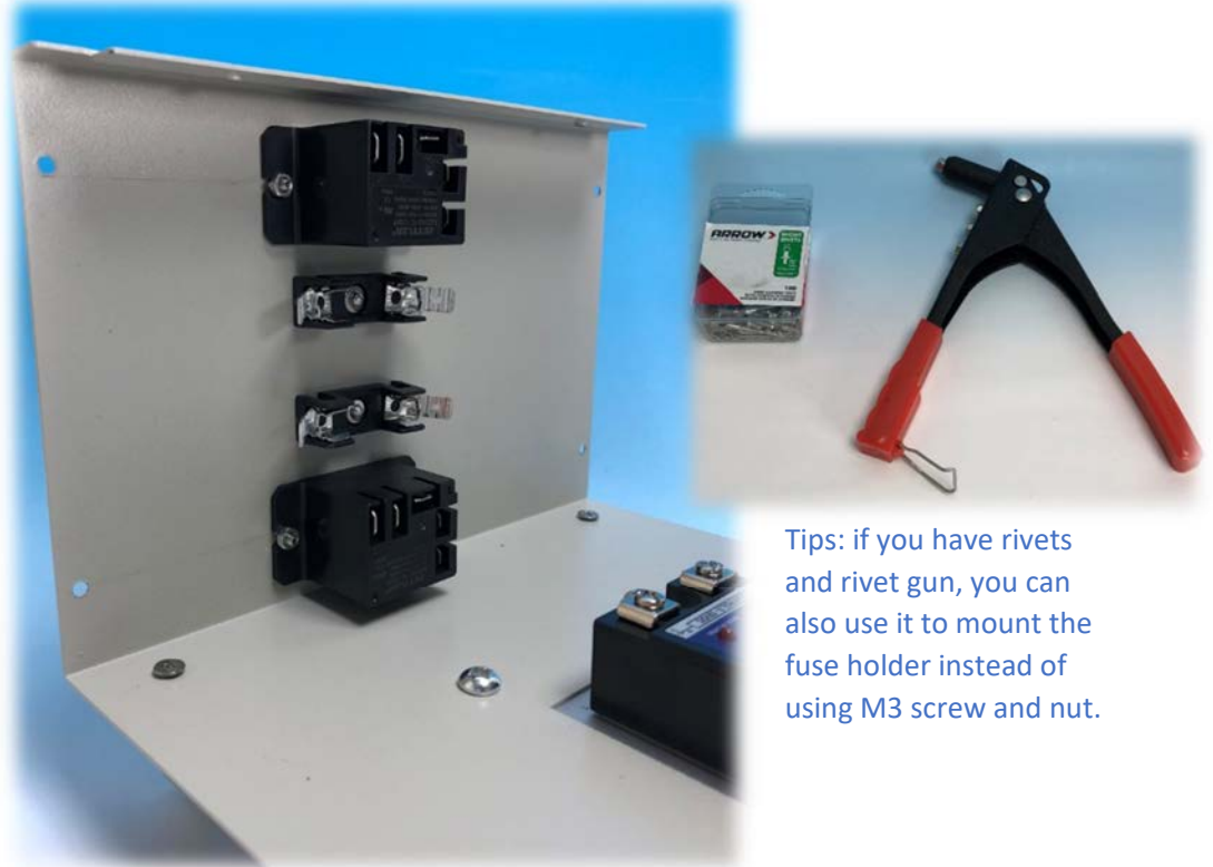
Figure 11. Inside view (all nuts should be installed inside).
