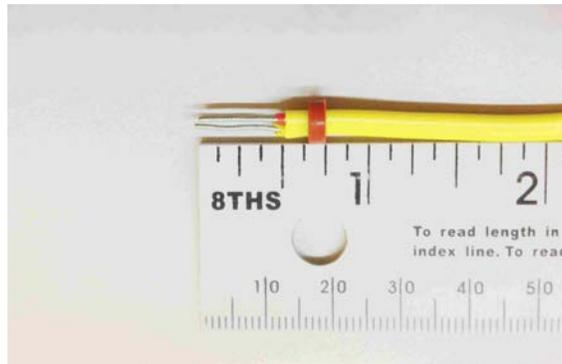
2. Put the red ring and clear ring (included with the connector) onto the cable and screw the wires to the female and male connectors.
