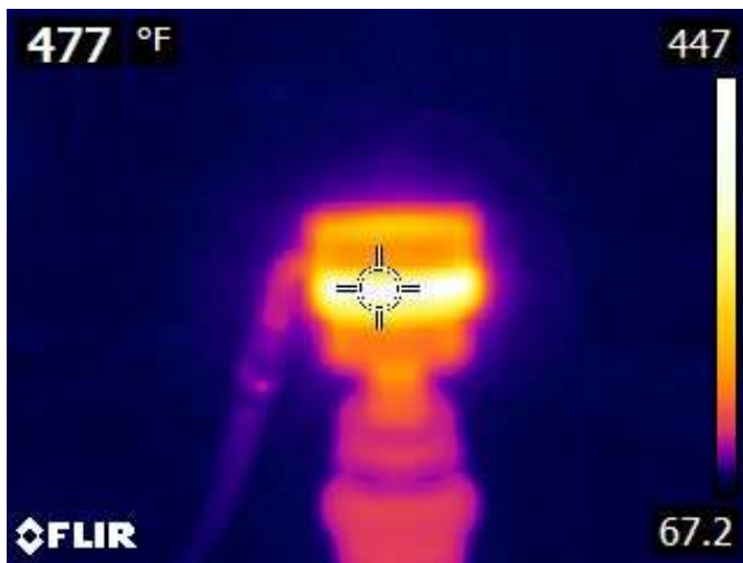
Fig 2b. An Infrared thermal image of Auber flat coil/universal nail assembly. SV = 600F. Side view. The temperature reading at the top left corner is from circle at the center.
