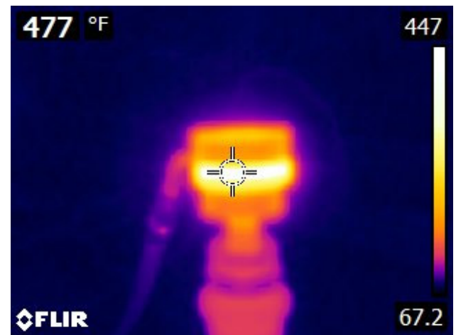
Figure 3(b). An Infrared thermal image of Auber flat coil/universal nail assembly. SV = 600F. Side view. The temperature reading at the top left corner is from circle at the center.
