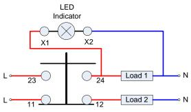
The indicator is on when the button is pushed in
