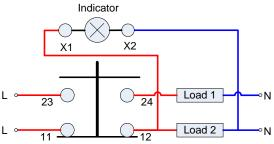
The indicator is on when the button is not pushed in
