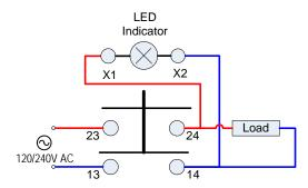
The indicator is on when the switch is closed
