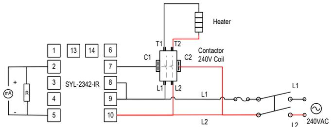
Figure 11. Control a heater in a 240 V system.
