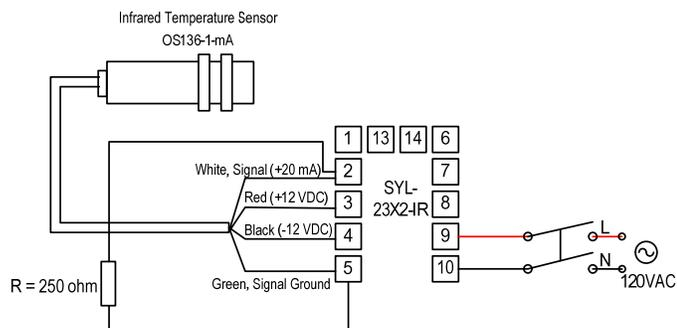
Figure 12. Wire an OS136-1-mA non-contact infrared sensor to SYL-2342-IR controller.
