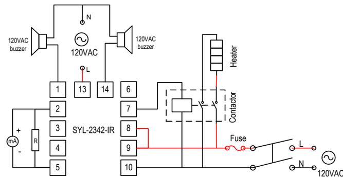
Figure 7. Wire a SYL-2342-IR with an external contactor to control a heating element. This is a typical wiring for oven or kiln.
