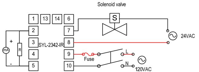
Figure 8. Wire a SYL-2342-IR with a solenoid valve. This is a typical wiring set up for a 24 V gas valve, hot water valve, or a contactor with 24 V coil voltage.
