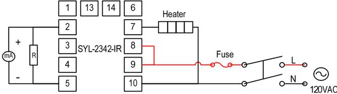
Figure 6. SYL-2342 or SYL-2342P control the heater directly by the internal relay of the controller. The heater must consume less current than the internal relay's maximum rating (7 A at 240VAC and 10 A at 120VAC).
