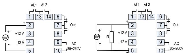
Figure 1. Wiring diagram of transducer with voltage signal (left) and milliamp current signal (right).
