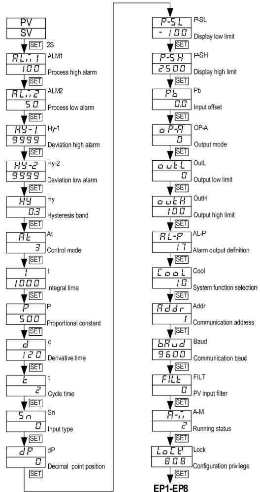
Figure 4. System setup flow chart
