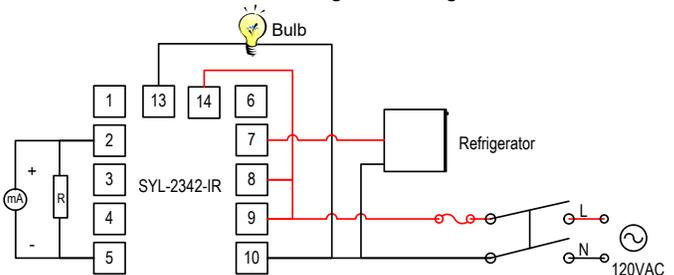
Figure 9. Connect both heating and cooling devices to SYL-2342-IR.
