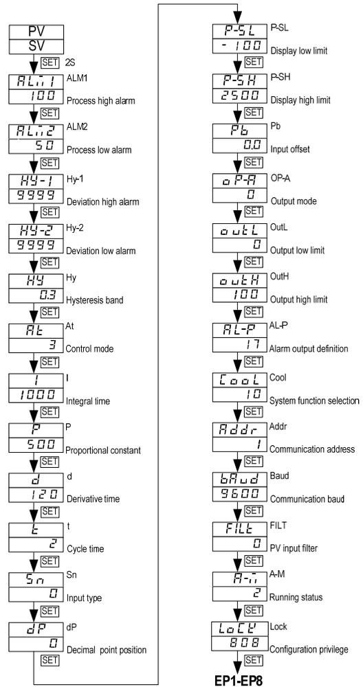
Figure 4. System setup flow chart
