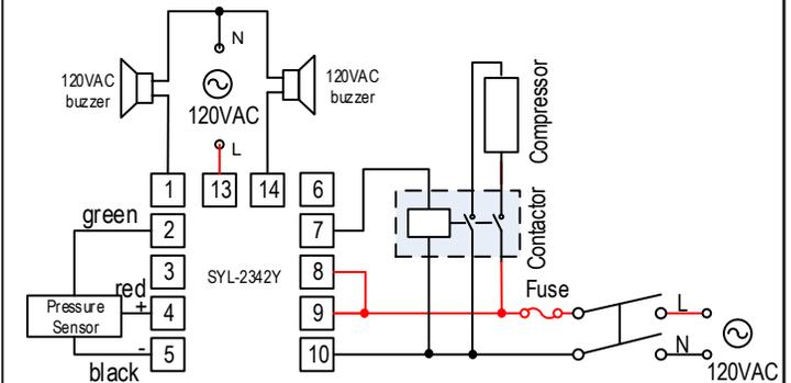
Figure 6. SYL-2342Y with external relay output.
