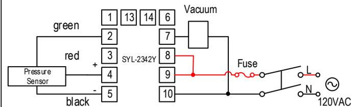
Figure 5. SYL-2342Y controls the vacuum directly by the internal relay of the controller. The vacuum must consume less current than the internal relay's maximum rating.
