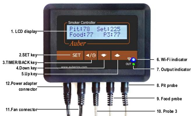
Figure 1. Front panel of a SYL-3615 controller.
