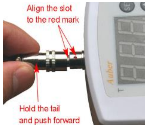
Figure 4. Install the Sensor
