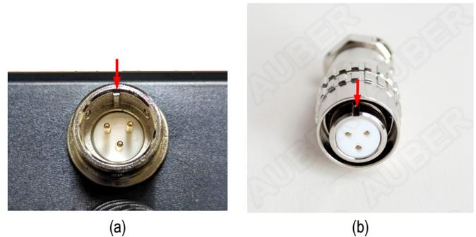
Figure 6. (a) The key on the male connector on the controller. (b) The notch on the female connector on the sensor cable.
