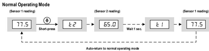
Figure 2. How to check the Sensor 2 reading.
