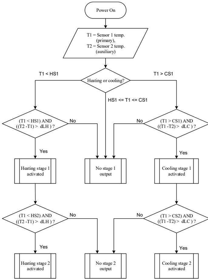
Figure 4. The operating logic of TD340.
