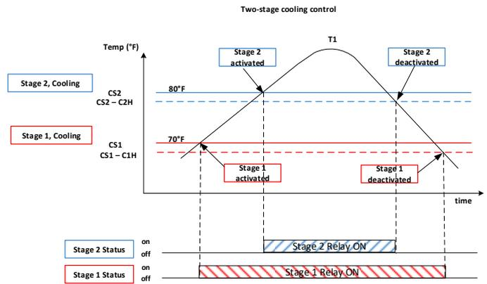
Figure 5(a). Relay output during two-stage cooling control.
