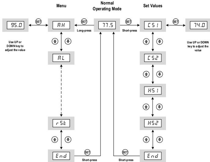
Figure 3. How to access the set values and the parameters in the menu.
