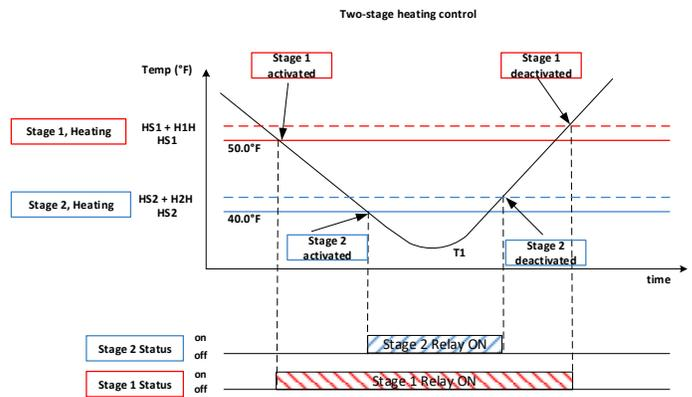
Figure 5(b). Relay output during two-stage heating control.
