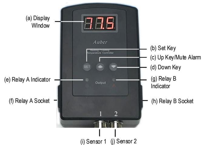
Figure 1. The front panel of TD340.
