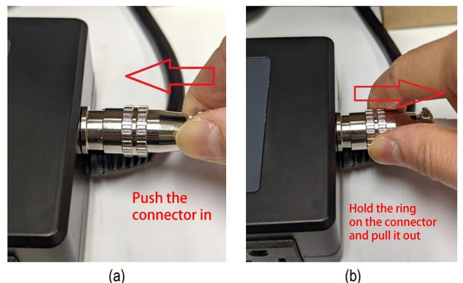
Figure 7. (a) To plug in the sensor connector, push from the connector behind the ring. (b) To unplug a sensor connector, hold the ring on the connector and pull it out.
