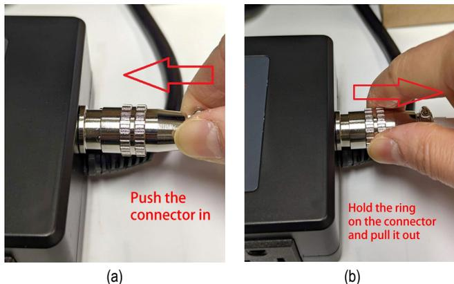
Figure 8. (a) To plug in the sensor connector, push from the connector behind the ring. (b) To unplug a sensor connector, hold the ring on the connector and pull it out.
