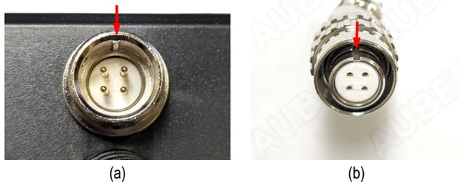
Figure 7. (a) The key on the male connector on the controller. (b) The notch on the female connector on the sensor cable.
