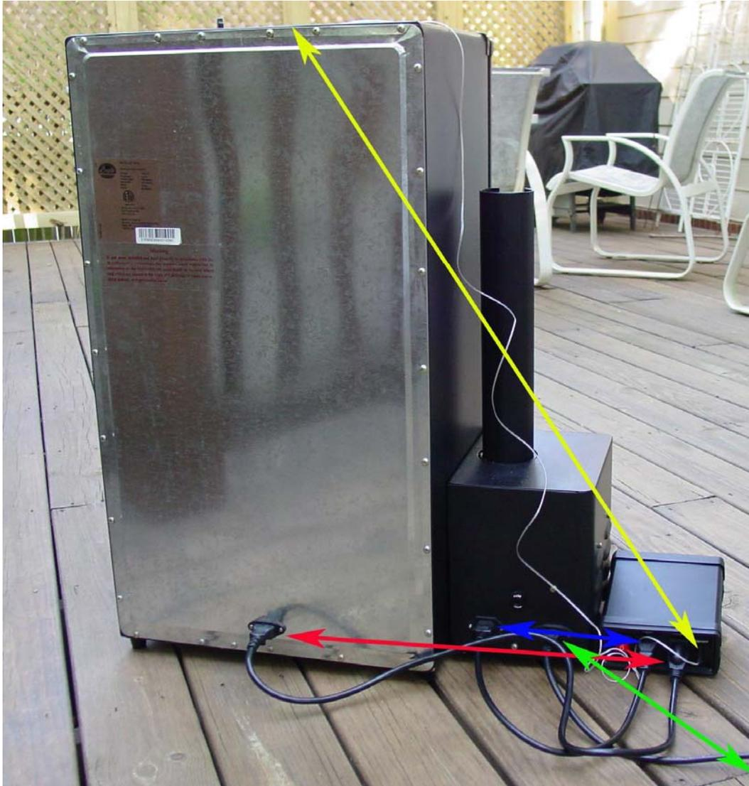
Fig 4. Power connection of the controller and smoker.
