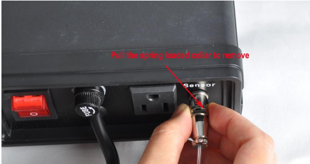
Figure 5. How to remove the sensor.
