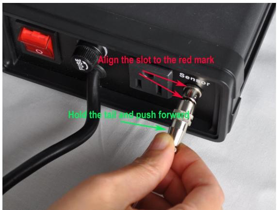
Fig 3a. How to install the sensor.
