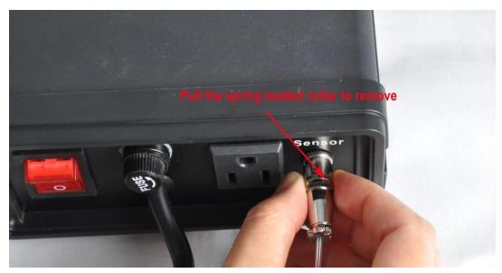
Fig 3b. How to remove the sensor.
