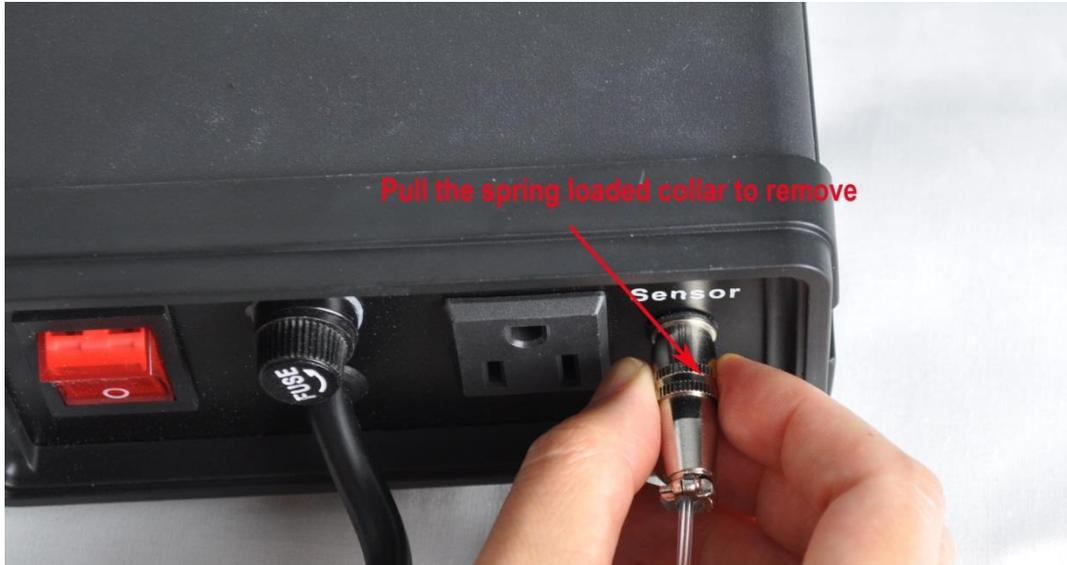
Figure 4. How to remove the sensor.
